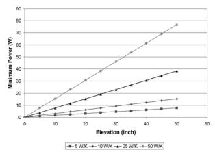
the delay in start-up is significant, the rise in temperature at the heat source may result in the maximum design temperature being exceeded on sensitive electronics. In the case of zero gas, the minimum temperature difference required across the wick is zero. As gas is added, a finite temperature difference must be established before circulation can begin.
