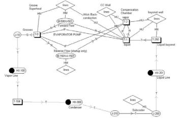
The goal of the analyses was to determine the effect on start-up of significant evaporator mass, adverse tilt and noncondensible gas in the loop. This required a transient hydrodynamic simulation to which the modeling of the compensation chamber and the evaporator wick were paramount.
