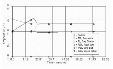
Figure 6: Startup with 10 Watt Load 24 lbs mass, no tilt, no gas
