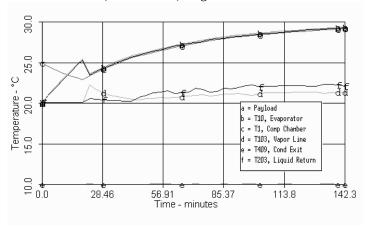
conductance shows that 10 watts is insufficient in offsetting the wick back conduction and subcooling associated with 25 inches of adverse tilt.
