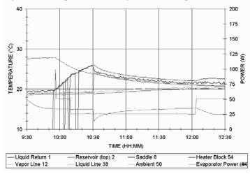
Figure 12: Reverse Flow at LHP Startup (Test Data)
