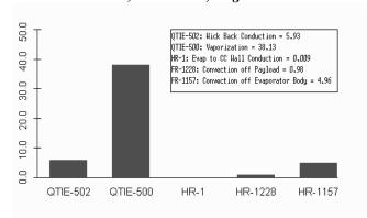
Figure 10: Startup with 10W Load, Mass and Gas 24 lbs. Mass, No Tilt, 0.0038 gm-moles Gas
