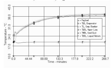
Figure 9: Startup with 50 Watt Load, Heat Flow Summary No mass, 25" adverse, no gas
