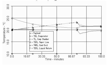
Figure 7: Startup with 10 Watt Load No mass, 25" adverse, no gas
