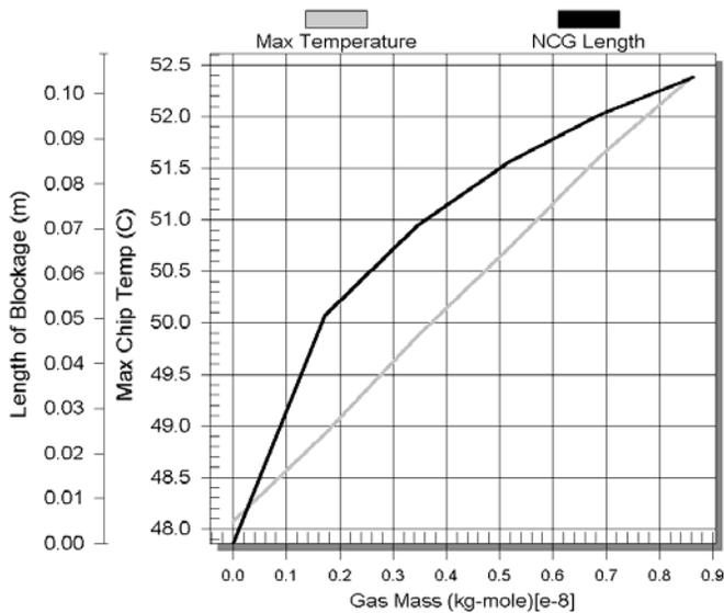
**Figure 4: Effect of Degradation via NCG Generation**
