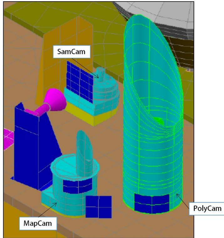
*Figure 1: OSIRIS-REx Camera Suite (OCAMS) Thermal Desktop models*
