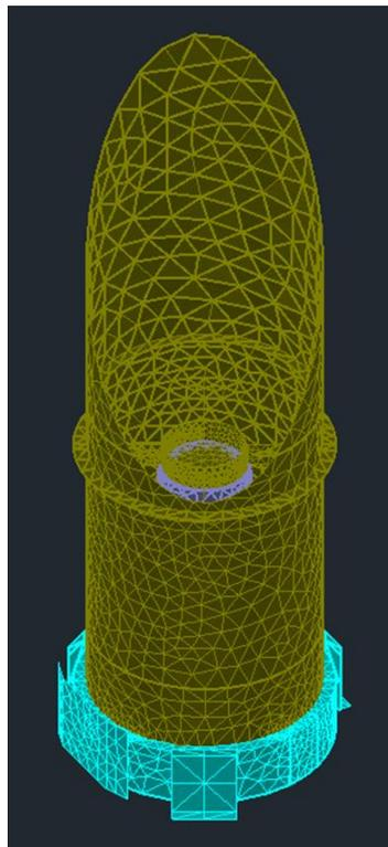
*Figure 2: Detailed Thermal Desktop model of PolyCam*
